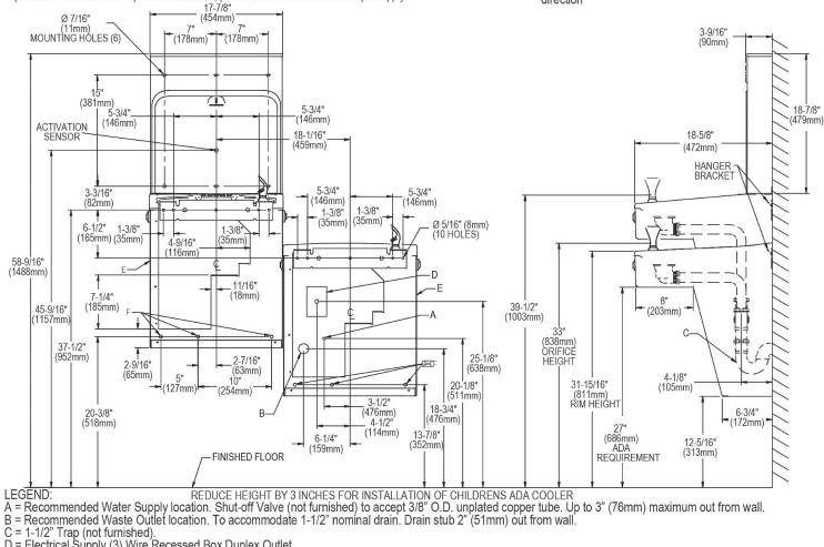
D = Electrical Supply (3) Wire Recessed Box Duplex Outlet.
